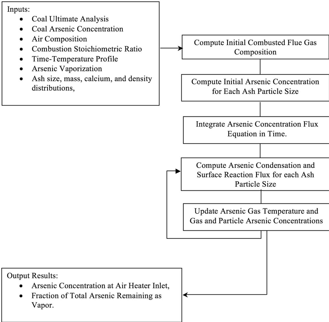
Figure 3: Arsenic model flow diagram.
